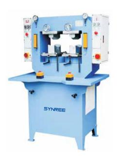
※ This machine is suitable for moulding the mid-sole for lady shoes/man shoes,to make it attaching the last for lasting.
